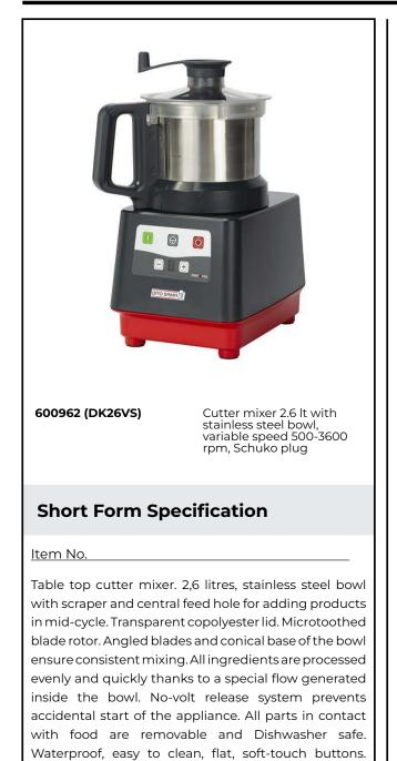
Variable speed with 9 levels (500 to 3600 rpm) for extra
